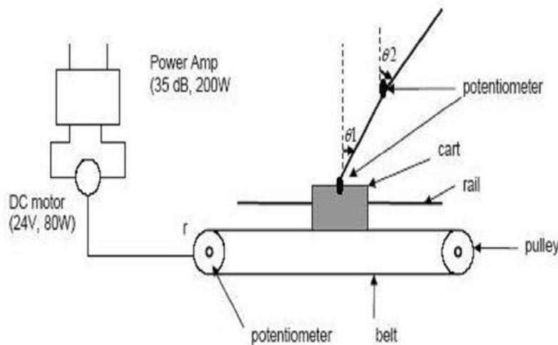
**Figure.1.**Diagram of the Double Inverted Pendulum System
