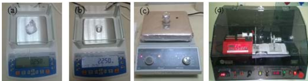
Figure 4.9. Preparation and electrospinning process of 10 wt. % PAN polymer content solution. (a) 0.250 gr of PAN, (b) 2.250 gr of DMF, (c) solution of PAN and DMF on the magnetic stirrer, (d) electrospinning process
