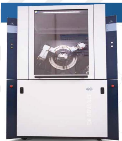
Figure 4. 31. XRD, Bruker advanced X-ray solutions D8 (S.U, Iltek)
