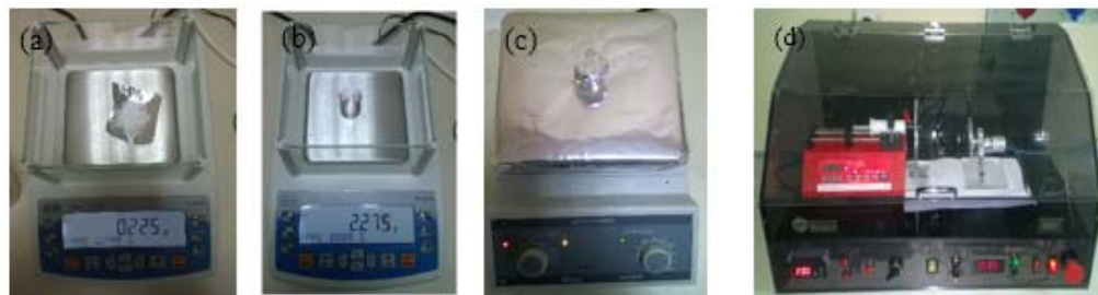
Figure 4.8. Preparation and electrospinning process of 9 wt. % PAN polymer content solution. (a) 0.225 gr of PAN, (b) 2.275 gr of DMF, (c) solution of PAN and DMF on the magnetic stirrer, (d) electrospinning process
