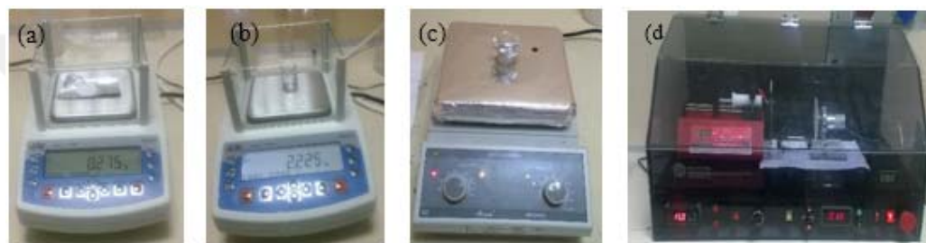
Figure 4.10. Preparation and electrospinning process of 11 wt. % PAN polymer content solution. (a) 0.275 gr of PAN, (b) 2.225 gr of DMF, (c) solution of PAN and DMF on the magnetic stirrer, (d) electrospinning process
