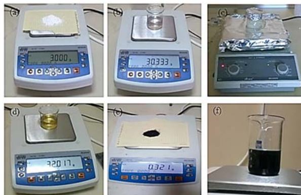
Figure 4.21. Weighing of chemicals and preparation of electrospinning solution containing 1 wt. % of graphene NPs. (a) 3.00 gr of PAN, (b) 30.333 gr of DMF, (c) Steering of PAN/DMF mixture. (d) 32.017 gr of PAN/DMF solution after steering, (e) 0.32 gr of graphene NPs, (f) Mixture of PAN/DMF/graphene NPs after steering process
