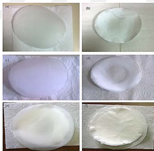
Figure 4.28. Pictures of pure PAN/DMF/Silica NPs electrospun nanofibers. (a) 1 wt. % Silica NPs and 15 kV, (b) 1 wt. % Silica NPs and 20 kV, (c) 3 wt. % Silica NPs and 15 kV, (d) 3 wt. % Silica NPs and 20 kV, (e) 5 wt. % Silica NPs and 15 kV, (f) 5 wt. % Silica NPs and 20 kV. All the other variables remained constant
