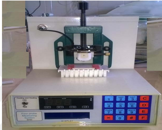
Figure 4. 33. Four-point probe device (ENTEK Elk. FPP-460)
