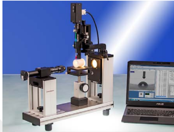
Figure 4.32. OCA15EC with single-direct dosing system ( http://www.dataphysics.de )
