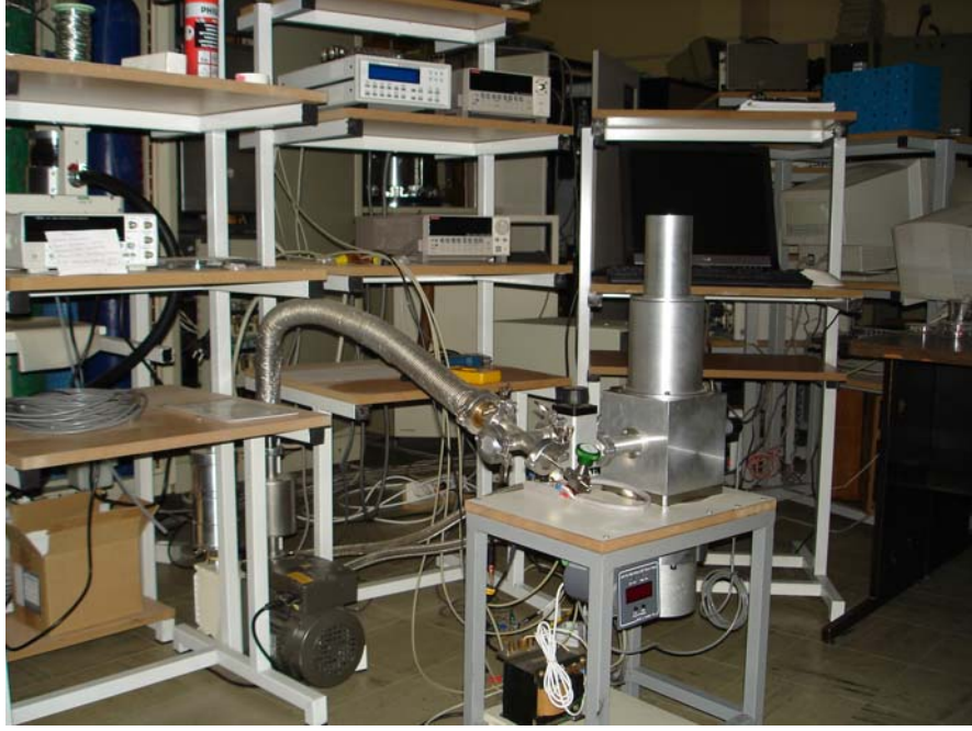
Şekil 3.11 CTI-Cyrogenics Cyrodyne Refrigerator System.
